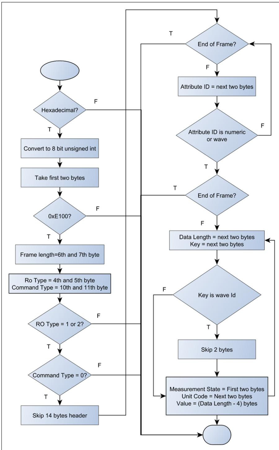
Figure 4. Data decoding
