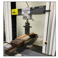
Figure 5. Set up for the 3-point flexure bending test
